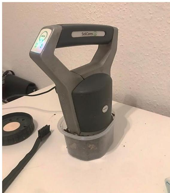
**Fig. 1. The Near Infrared (NIR) AgroCares Scanner in use (1300–2600 nm). The scanner has one button for switch on and off and for starting the scanning process. There is also a reset option on the side of the device. A white and a yellow puck is used for calibration. There is a brush for cleaning the scanner surface.**
