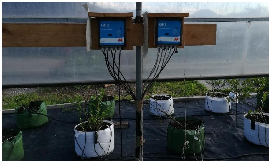
**Fig. 2. Data loggers for growing substrate water content and temperature measurements at the experimental set-up for highbush blueberry (Stražar, 2022).**
