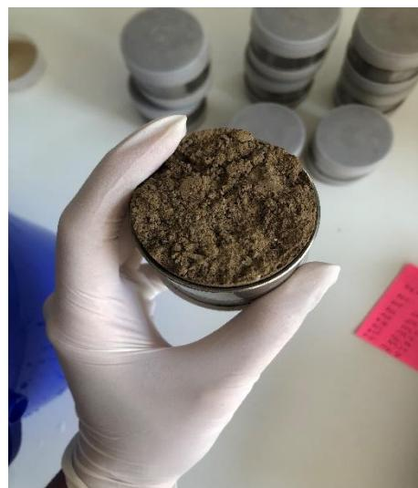
**Fig. 2. Soil sample for measurement soil moisture by the gravimetric method under laboratory conditions (Botkova, 2023).**
