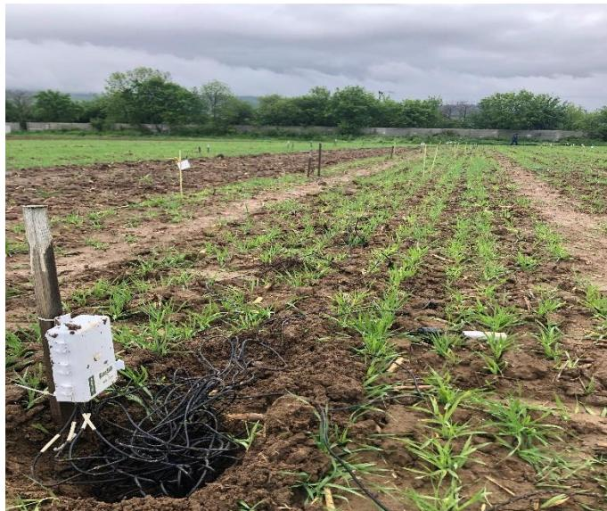
**Fig. 1. Installation of sensors at the Malanta experimental site (Botkova, 2023).**
