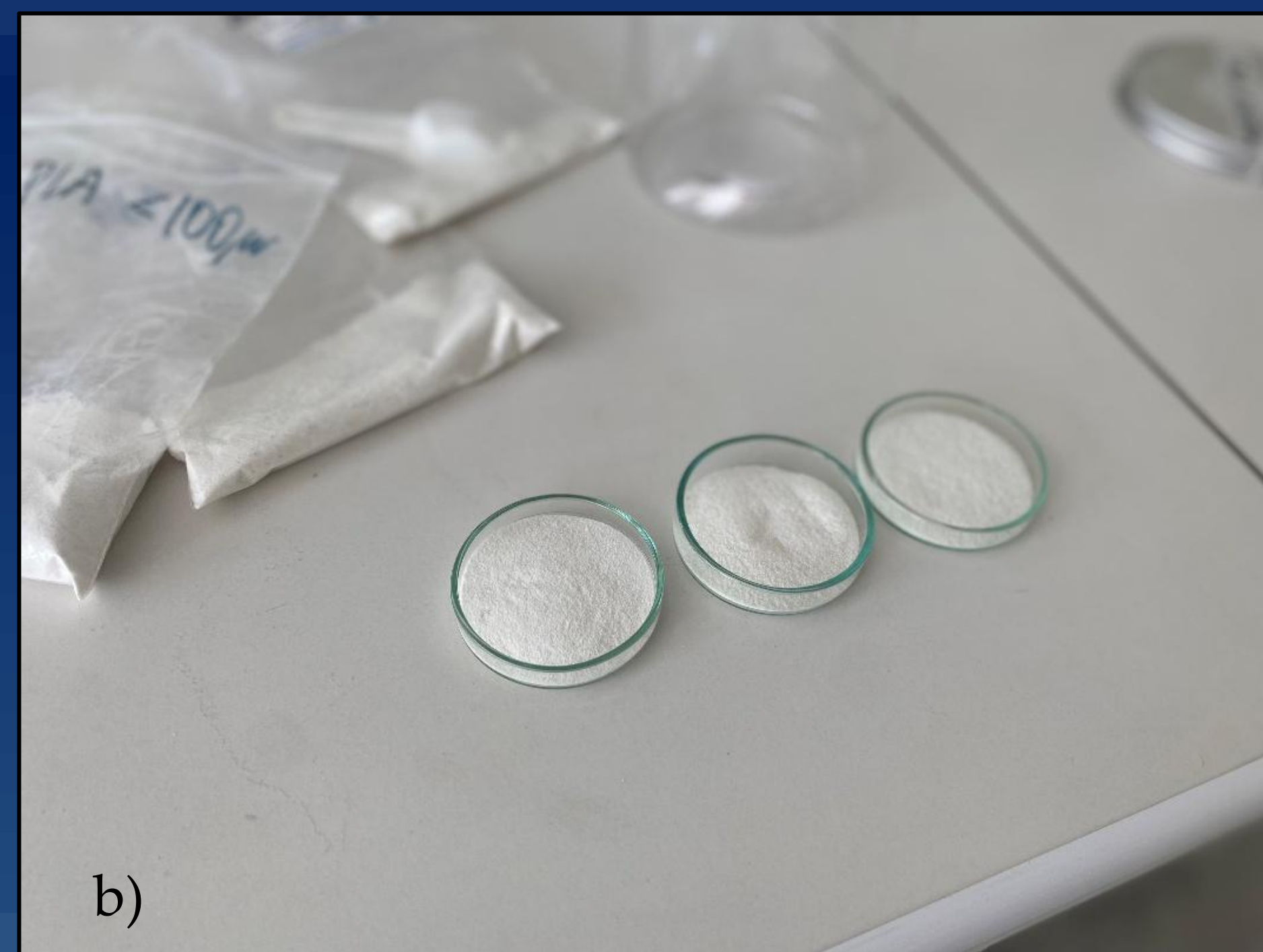
Figure 1 a) KSAT equipment for saturated hydraulic conductivity measurement, b) disparate fractions of polylactic acid (PLA): from right small <100, medium 100–200 and large >200 \mu\text{m} .
