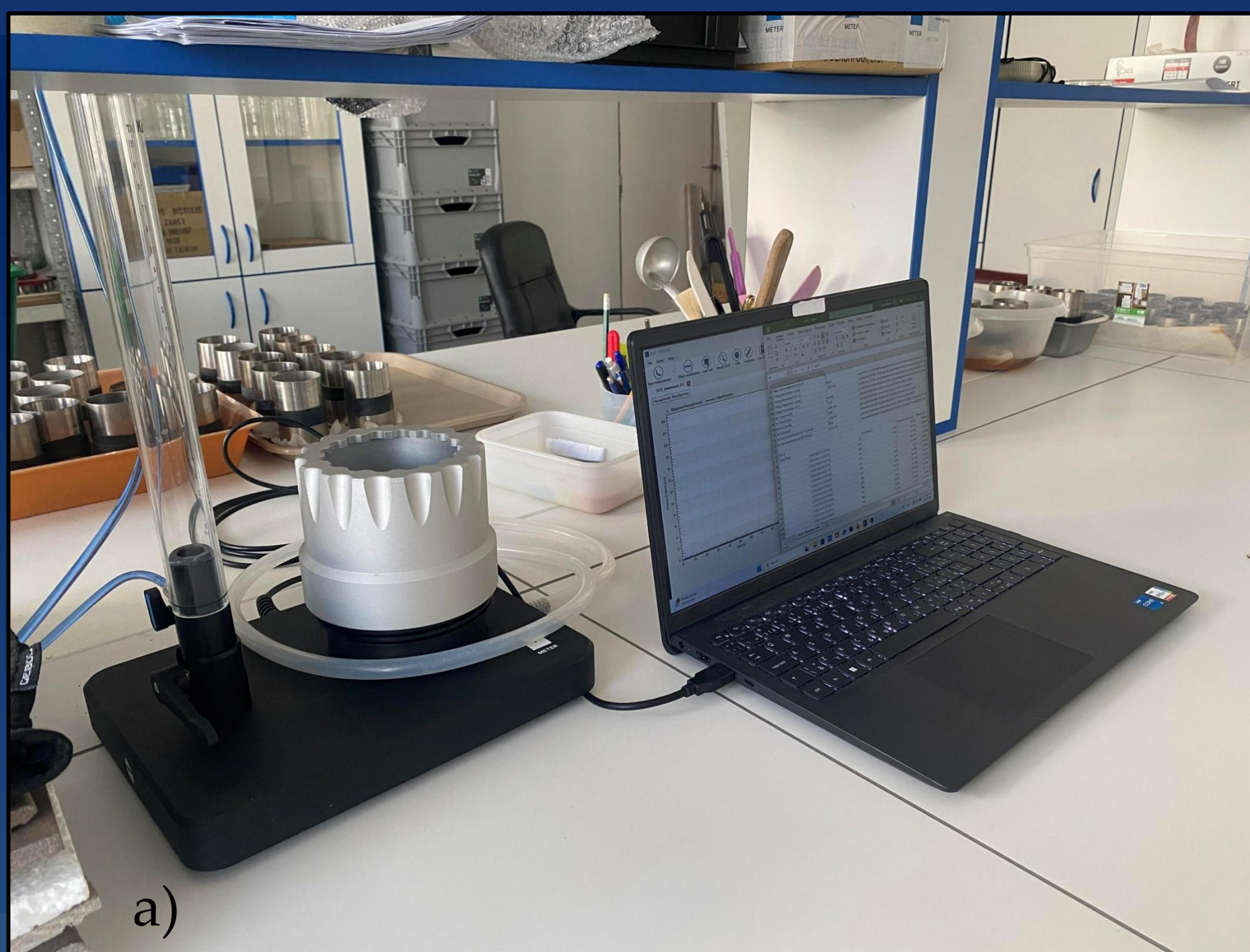
Figure 1 a) KSAT equipment for saturated hydraulic conductivity measurement, b) disparate fractions of polylactic acid (PLA): from right small <100, medium 100–200 and large >200 \mu\text{m} .
